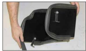
14. Install the edge trim onto the heat shield as shown.
