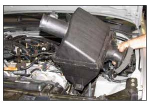
10. Pull firmly on the airbox to dislodge it from the mounting grommets and remove it from the vehicle. NOTE: K&N Engineering, Inc., recommends that customers do not discard factory air intake.
