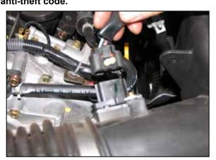
2. Disconnect the mass air sensor electrical connection and unhook the harness from the airbox.
