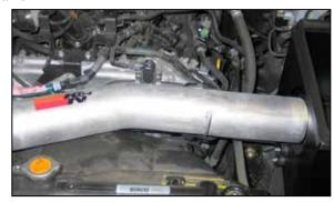
22. Install the K&N<sup>®</sup> intake tube into the silicone hose at the throttle body and align with the tube mounting bracket installed in step #16. Secure with the provided hardware and hose clamp.
