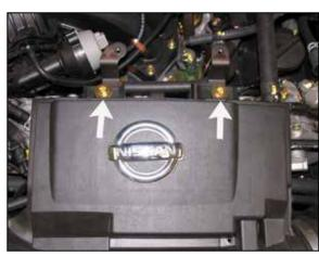
5. Remove the two bolts shown which secure the stock intake tube to the engine.
