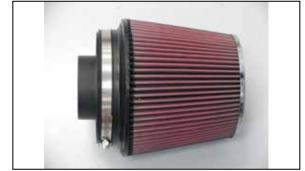
24. Install the filter adapter into the air filter as shown and secure with the provided hose clamp.
