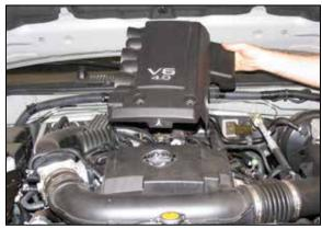
4. Lift firmly on the engine cover to dislodge it from the mounting grommets, and then remove the cover from the engine as shown.
