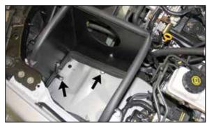
18. Install the heat shield assembly into the vehicle and secure with the provided hardware.
