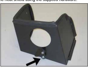
16. Attach the provided "C" bracket (070093) to the rubber mounted studs installed in the previous step using the provided hardware.
