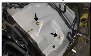
11. Remove the two airbox mounting studs shown from the inner fender.
