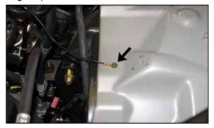
17. Remove the bolt, which secures the ground strap to the inner fender.
