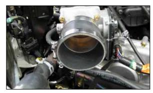
19. Install the silicone hose (084055) onto the throttle body and secure with the provided hose clamp.
