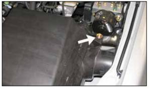
9. Remove the airbox retaining bolt shown.
