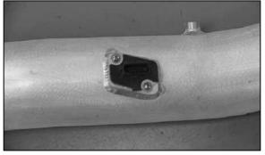
21. Install the mass air sensor into the K&N<sup>®</sup> intake tube and secure with the screws removed in step #20.
