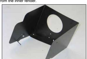
12. Install "L" Bracket (#07805) onto the heat shield with the provided hardware.
