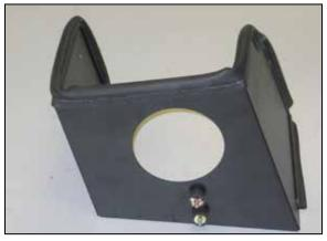
15. Install the provided rubber mounted studs onto the heat shield using the supplied hardware.
