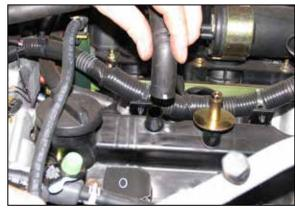
6. Using pliers, loosen the spring clamp which secures the crankcase vent hose to the valve cover and then remove the hose from the valve cover as shown.
