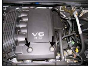
3. Remove the two bolts shown, which secure the engine cover.
