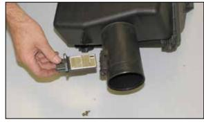
20. Remove the two screws, which secure the mass air sensor to the stock airbox and then remove the mass air sensor from the airbox.
