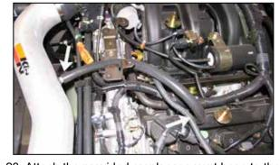
23. Attach the provided crank case vent hose to the valve cover and  $K\&N^{\otimes}$  intake tube as shown and secure with the provided hose clamps.
